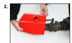
Ensure that the handle on the hitch is fully down, pass the cover over the hitch until the lock opening is positioned beyond the handle.
